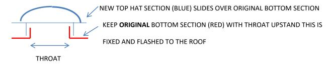
MEASUREMENT WE REQUIRE IS THE RED UPSTAND **EXTERNAL DIMENSION** OF THE THROAT TO BE ABLE TO MANUFACTURE BRAND NEW TOP HAT.
